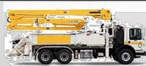
Concrete Pump 16 pcs
