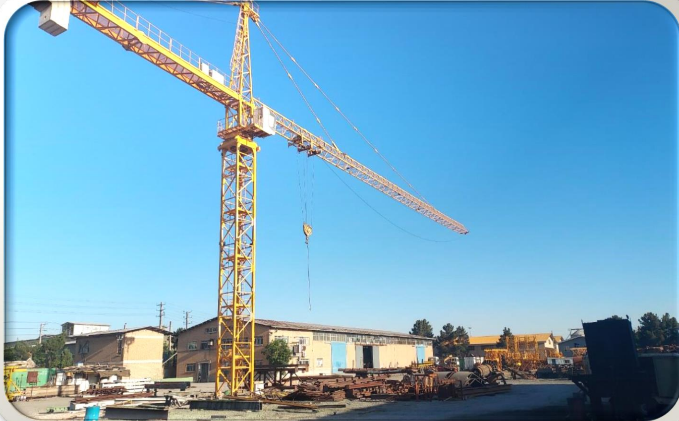
Zoomline Tower Crane 16 tons With height of 25 M. and flash duration 70 M.
